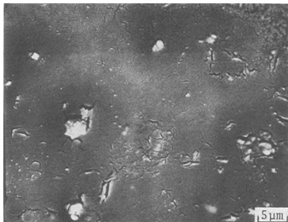
Figure 1 SEM micrograph of Fe-10 at% Si-15 at% B alloy glass aged for 30 sec at 721 K.
